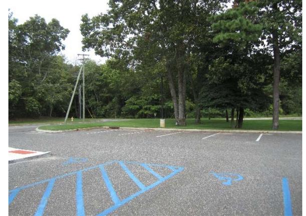
Parking spots in front of the building can be replaced with porous asphalt to capture and infiltrate stormwater. The sidewalk between two buildings can be replaced with porous concrete to capture roof runoff. Installing a rain garden adjacent to the building can capture, treat, and infiltrate roof runoff. A preliminary soil assessment suggests that more soil testing would be required before determining the soil's suitability for green infrastructure.
