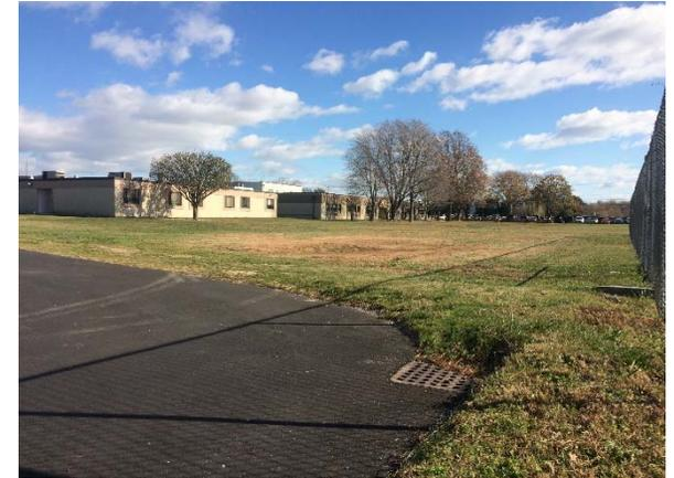
Installing a rain garden adjacent to the north corner of the school can capture, treat, and infiltrate roof runoff. Another rain garden can be installed in the turfgrass area southwest of the school and can treat runoff generated by the parking lot. A preliminary soil assessment suggests that the soils have suitable drainage characteristics for green infrastructure.
