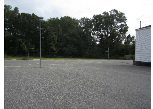
Parking spots in front of the building can be replaced with porous asphalt to capture and infiltrate stormwater. Installing a rain garden in the turfgrass area northeast of the church can capture, treat, and infiltrate parking lot runoff. A preliminary soil assessment suggests that more soil testing would be required before determining the soil's suitability for green infrastructure.
