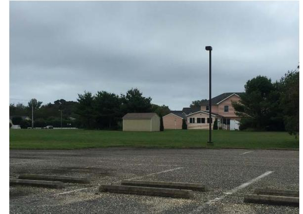
Parking spots south of the church can be replaced with porous asphalt to capture and infiltrate stormwater. Installing a rain garden in the turfgrass area southeast of the parking lot can capture, treat, and infiltrate parking lot runoff. A preliminary soil assessment suggests that the soils have suitable drainage characteristics for green infrastructure.
